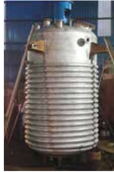
Limpet Coil Reactor
