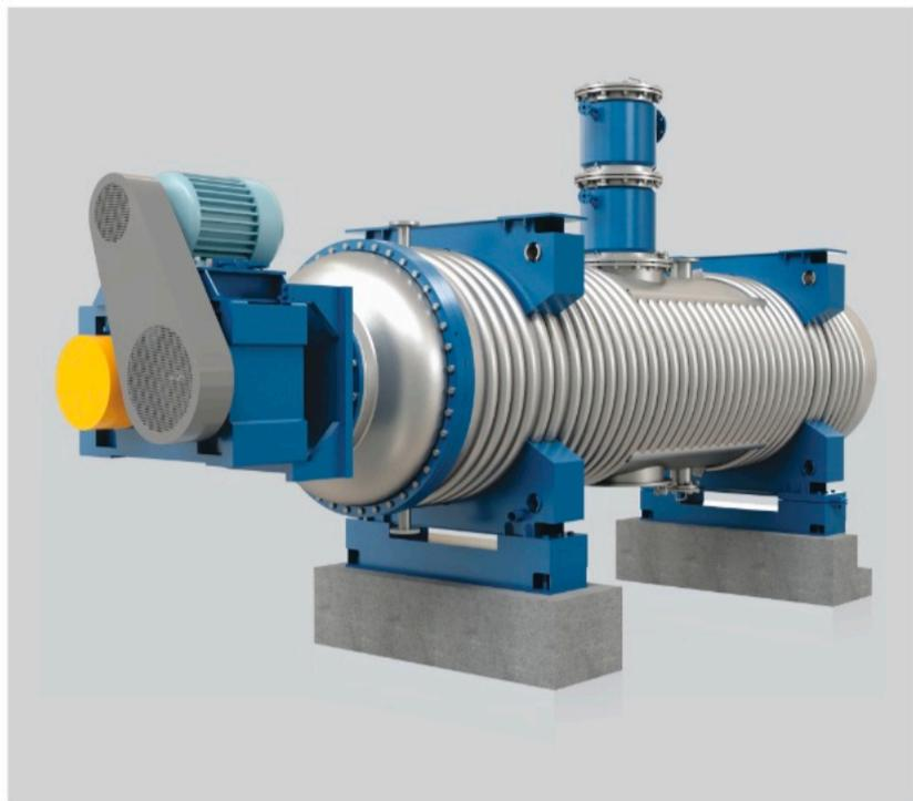
Rotary Vacuum Paddle Dryer(RVPD) offers a versatile, clean, simple and effective Process Solution for Vacuum Drying at Low Temperatures, Extraction of useful Liquids, Solvent Distillation / Recovery, Reaction, Crystallization, Process commencing with either Slurries or Pastes or Wet Cake, in Batch Operation carried out by indirect heating and often under Vacuum.
